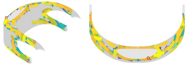
CFRP patches for structural reinforcement placed on the base CFRP structure of the hip component of a lower-limb exoskeleton
